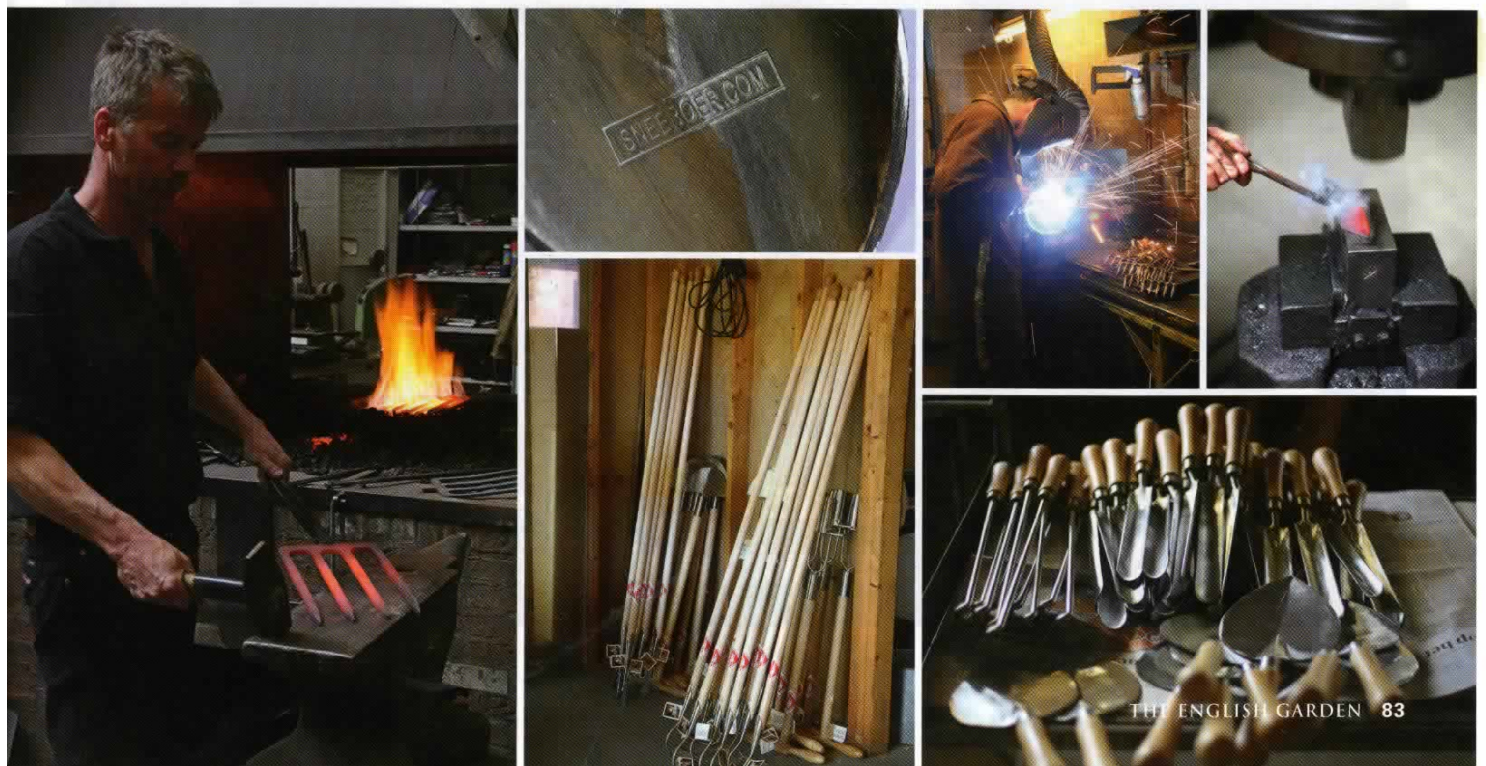
LEFT Fired for strength. ABOVE Keeping it in the Sneeboer family (Jaap: front row, third from right). BELOW, CLOCKWISE FROM LEFT Frank, with a fork glowing from the embers; branding on a trowel; welding on rake tines; using the 1920's sledgehammer; finished tools; the last stage - attaching ash handles.
