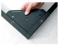
4. Check that you are happy with the positioning of the framework within your plot. Then using a corner connector plate (ref. 20) make absolutely sure that the joints are perfectly square as the ultimate success of the assembly relies upon this! Diagonals can also be measured. When both are equal the frame is square.
