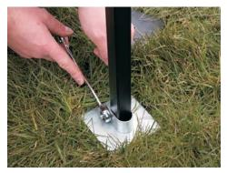
23. Using two 13mm spanners lock the foot plates (ref. 13) in place on the door support upright and the hinge upright using foot plate clamps (ref. 12). This prevents uprights sinking. After this level out all horizontal bars using a spirit level and soft mallet. Lock off all remaining foot plate clamps once this is done.
