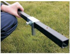
2. Decide where the door(s) should go (see step 9) and slide a T-joint (ref. 6) onto the appropriate horizontal bar(s) (ref.14). Ensure that the orientation of the parts is as shown, with the threaded holes facing upwards and the locking bolt on the T-joint facing into the cage.
