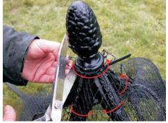
26. Slide the fitted roof net down over the fnial and align the seams with the curved bars. Using net ties (ref. 27) secure the net around the base of the fnial and also around the curved bars as the red arrows show. Trim off the ends of the ties and also any untidy stray netting.
