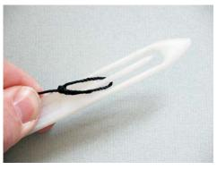
42. Load the whipping needle with the whipping twine supplied by frst tying one end to the needle.
