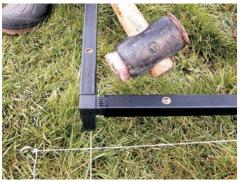
8. Once all of the marking out with string is complete, carefully dismantle the horizontal bar framework leaving connected only bars that can exist as a complete square unit (see step 13 for reference). Note that the threaded holes in the horizontal bars always face upwards.
