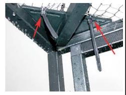
39. Using net ties (ref. 27) passed through the slots provided in the connector plates, secure the ftted roof net(s). Then using more net ties (approximately 1 every 30cm) work your way up the curved roof support bars (ref. 24) and secure the net to the curved bars along the net's seams.
